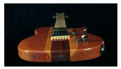
The battery compartment is located on the edge of the guitar above the bottom strap stud. The battery is held by and connected by the cover: a cross-laminated block of cherry wood with the battery terminals screwed to it on top of sheet copper, which makes the connection from the battery to the 2 coiled wires inside the guitar. That way, there are no wires to pull out, stuff back in, or break off.
