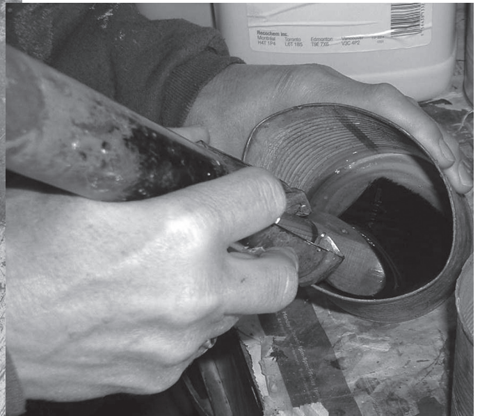
Figures 4 (left). A spin in the “slop” pail to remove the diesel fuel is step one in preparing a brush before using. The action is intense, but the bucket contains the spray. After taking a spin, the brush is rinsed in about a half inch of thinner (Figure 5, below), then spun again.
