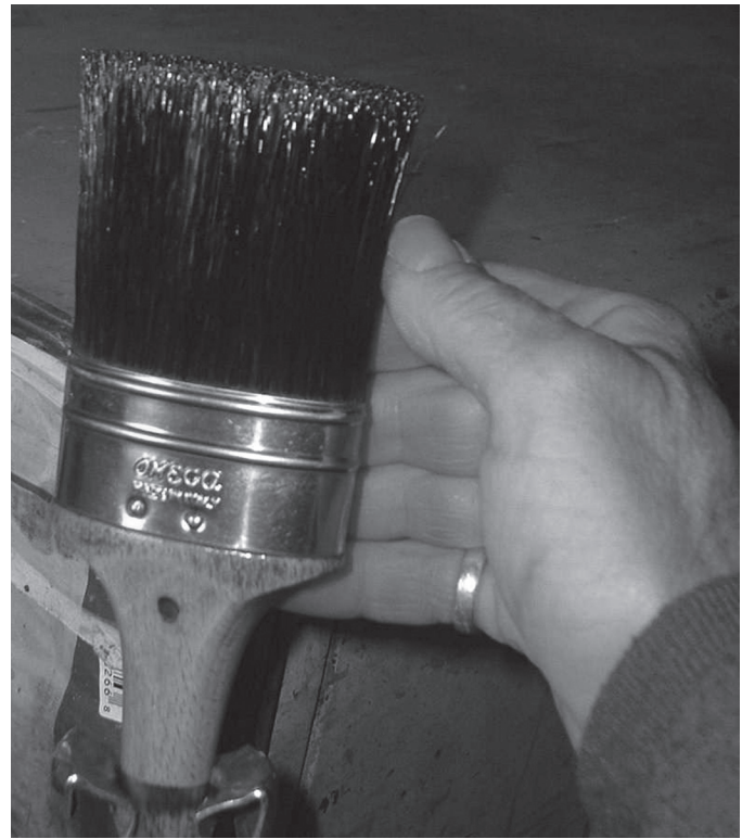
Figure 7. Paint brushes carry a lot of paint, so it's important to work the thinner up into the ferrule of the paint brush.
